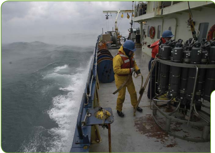
Figure 4. Scientists and crew aboard the UNOLS Intermediate Class R/V Oceanus prepare a Conductivity-Temperature-Depth instrument for deployment off Cape Hatteras. (Photo credit: C. Linder, Woods Hole Oceanographic Institution)
