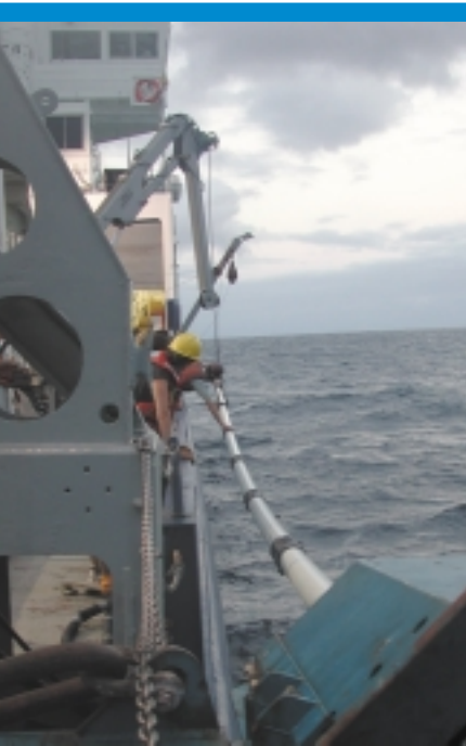
Figure 12. High-resolution studies of Earth's past climate rely on long, undisturbed records from ocean sediments. Oregon State University's long coring facility, here being deployed from the R/V Melville , can provide researchers with cores up to 20 m long, appropriate for studies of ice-age climate change over the last few hundred thousand years. Site selection was made based on seismic and swath bathymetric mapping just prior to coring. Photo courtesy of A. Mix, Oregon State University and M. Lyle, Boise State University.
