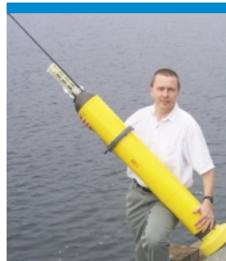
Figure 9. The Argo float program involves the deployment of several thousand freely drifting PALACE floats, which profile the oceanic temperature and salinity while moving with the circulation deep beneath the surface. In large numbers they are yielding a global picture of the evolving density structure of the ocean. Photo courtesy of S. Riser, University of Washington.
