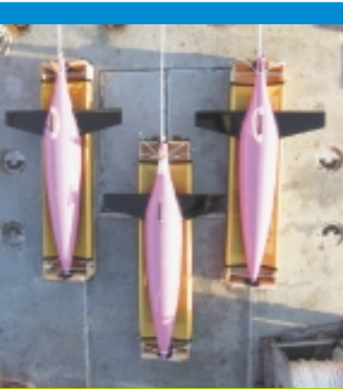
Figure 2. The Seaglider is one of several autonomous underwater vehicles that will permit oceanographers to measure hydrographic, chemical, and biological fields across the ocean. Seagliders can be launched from small boats and operate for a year without servicing. Instruments such as these free ships from routine sampling chores, permitting them to undertake tasks requiring special capabilities. Photo courtesy of C. Eriksen, University of Washington.
