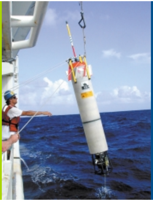
Figure 16. The Absolute Velocity Profiler, being deployed from the R/V Wecoma , as used in the Hawaiian Ocean Mixing Experiment. The lower end of the instrument contains sensors for measuring density, turbulent dissipation, and optical turbidity. The narrow dark band part way up the skin houses a two-axis electric field array, which measures relative velocity throughout the water column. Velocity measurements are made absolute by referencing the electric field to GPS and onboard by Acoustic Doppler Current Profiler (ADCP) measurements. Photo courtesy of J. Nash, University of Washington.
