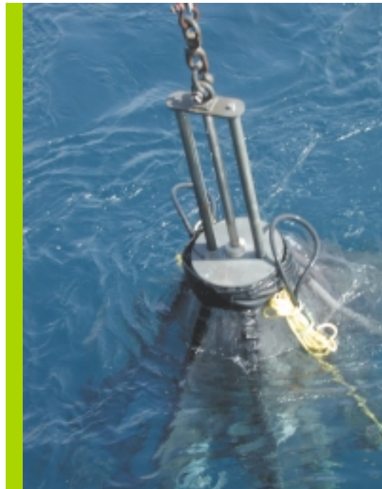
Figure 25. Oregon State University's multicore system, deployed from the R/V Melville , is recovered full of mud. This device lands gently on the seafloor, then penetrates about 50 cm before closing trap doors to safely recover multiple pristine samples of the sediment-water interface. Recovery often reveals living tube worms or shrimp—somewhat startled but essentially undisturbed. Such sampling devices offer a unique glimpse of life at the seafloor and the chemical transformations that occur as newly fallen biogenic debris is converted into the sedimentary record. Photo courtesy of A. Mix, Oregon State University and M. Lyle, Boise State University.
