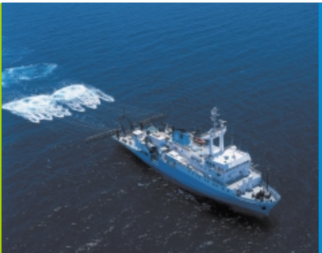
Figure 13. R/V Ewing shooting multichannel seismic profiles in the Gulf of Corinth. Photo courtesy of Lamont-Doherty Earth Observatory.
