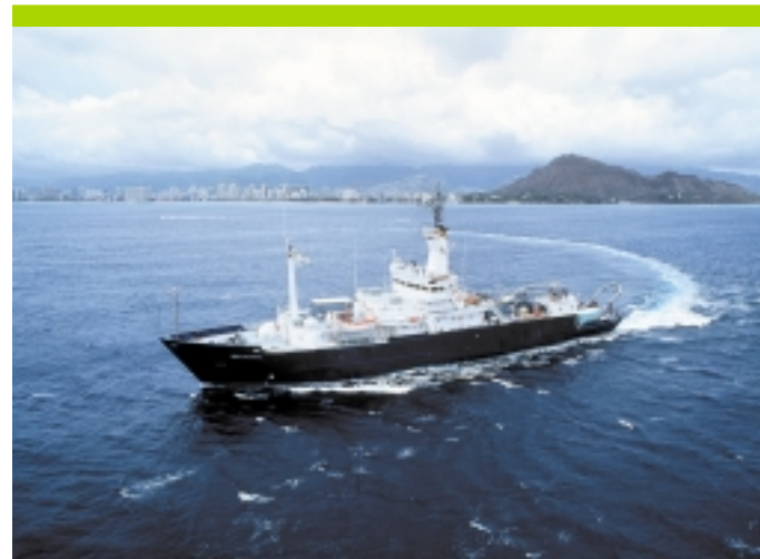
Figure 3. The Global Class R/V Melville , built in 1969 and re-engined, stretched, and upgraded in 1991.
