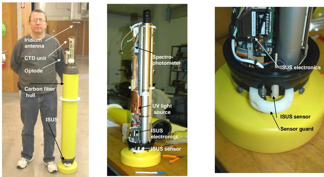
**FIGURE 1. The initial design of ISUS for a profiling float. In this version the sensor is located on the lower endcap of the float. The float is also equipped with an Aanderaa Optode dissolved oxygen sensor and uses Iridium communications.**
