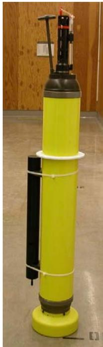
**FIGURE 3.** A mock-up of a profiling float with a Satlantic SUNA nitrate sensor unit attached. This design will be deployed and tested in the upcoming year.
