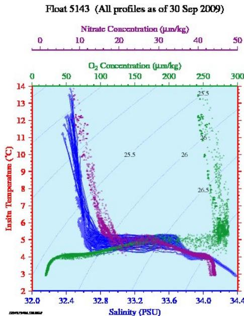
**FIGURE 4.** Top panel: Temperature, salinity, dissolved oxygen, and nitrate data from 81 profiles from UW profiling float number 5143 in the Northeast Pacific. The profiles were collected at 5-day intervals between August 2008 and September 2009 (the float continues to function normally through the end of 2009). Bottom panel: Salinity, dissolved oxygen, and nitrate plotted as functions of temperature from float 5143.
