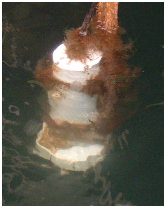
Fig 3. The C/T Sensor at the WHOI dock after three months deployment. Algae has colonized the support strut and clamps but the instrument itself has remained largely clear of fouling.
