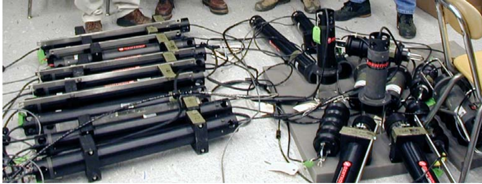
Figure 4. Immediately preceding the FRONT-3 deployment, project personnel programmed and exercised the Seaweb network and Seaweb server as an in-air network.
