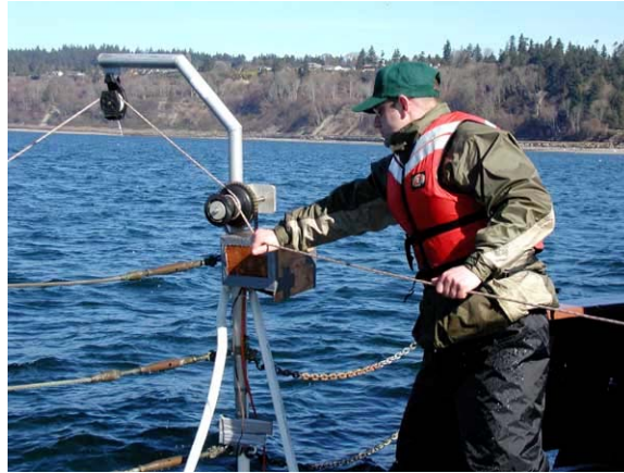
Figure 1: An OIP student participant helps gather CTD data on Puget Sound, WA. [Man uses winch to help pull CTD in from Puget Sound.]
