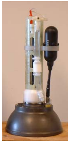
Figure 2. The head of a Webb/Apex float, showing a SeaBird CTD unit and a broadband hydrophone for an acoustic rain gauge. An Argo float with this ARG unit will be deployed late in 2003.
