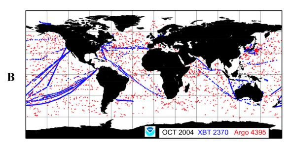
**Figure 3: (A)** Argo and XBT Near Real-Time Profiles Per Month; **(B)** Data Delivered in Real Time during October 2004 from Argo (4395 Profiles Typically to Over 1000m - Red Dots) and from the High density XBT Network (Temperature Only to Typically 750m - Blue Dots). Courtesy AOML.
