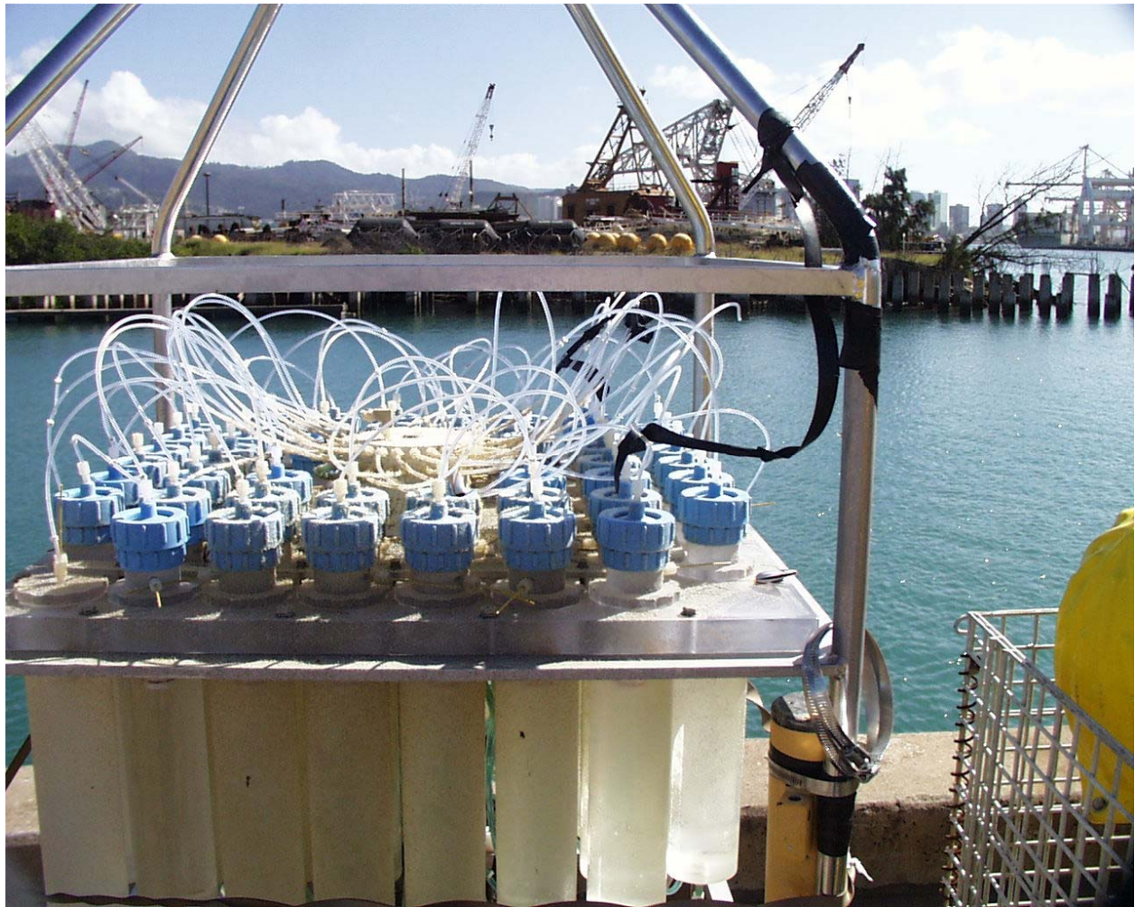
Figure 6. Pictures of the RAS before, with some of the major components - and after the deployment, a bit fuzzy with biofouling after three months exposure.
