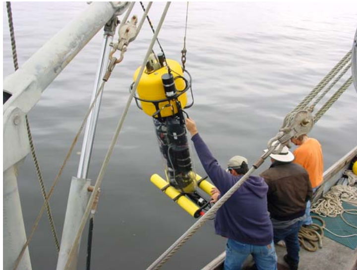
Figure 1. URI Scientists deploying the IOPC profiler with the newly developed APNA II nutrient analyzer payload in Monterey Bay from the R/V Shana Rae.
