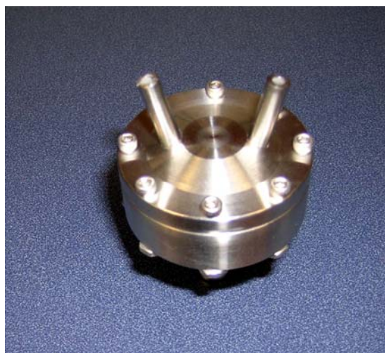
Figure 2: second generation prototype of TETHYS inlet, weighing approximately ½ kg in air, measuring approximately 10 cm in diameter.
