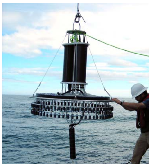
Figure 4. The Pelagic Imaging Mid-frequency Multibeam Sonar (PIMMS) being deployed.
