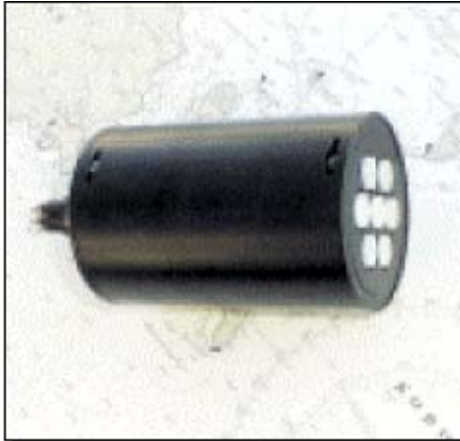
Figure 3. The irradiance sensor were incorporated into Glider science bays in 2006.
