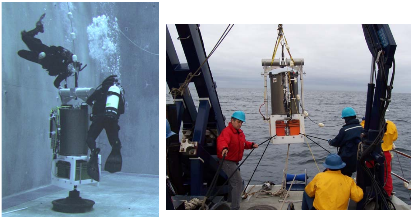
Figure 2. The 2G ESP being deployed in MBARI's test tank with divers inspecting the package (left), and the same instrument being deployed from the R/V Zephyr in Monterey Bay March 2006.
