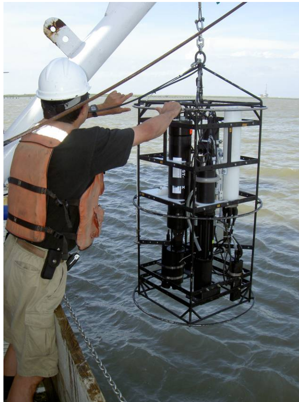
Fig.3. USM Instrument Frame With AC-9/AC-S and ECO-VSF3 Being Deployed in Gulf of Mexico for testing (Summer 2006).
