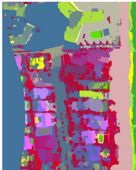
Fig. 17. Topographic Blobs Produced from Casi Data with Mean Shift Algorithm
