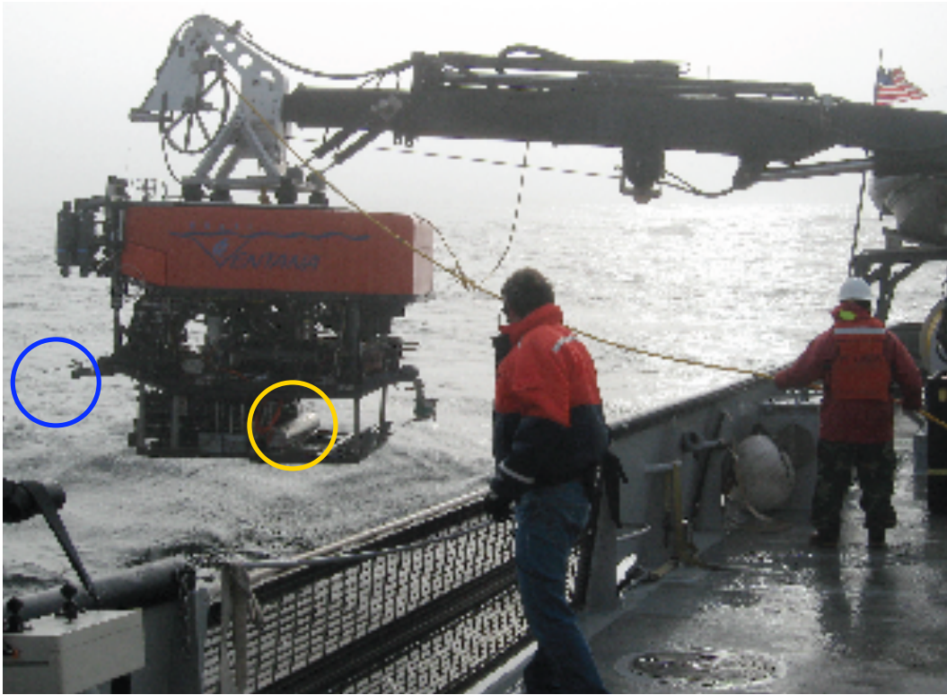
Figure 1. First field deployment of the in situ ICOS instrument on the ROV Ventana aboard the R/V Point Lobos on October 6 th , 2008. The instrument is housed inside a cylindrical titanium pressure housing positioned in the rear of the ROV (orange circle). The sampling wand, through which sample fluids are delivered to the membrane inlet on the housing, is in the port manipulator (blue circle).
