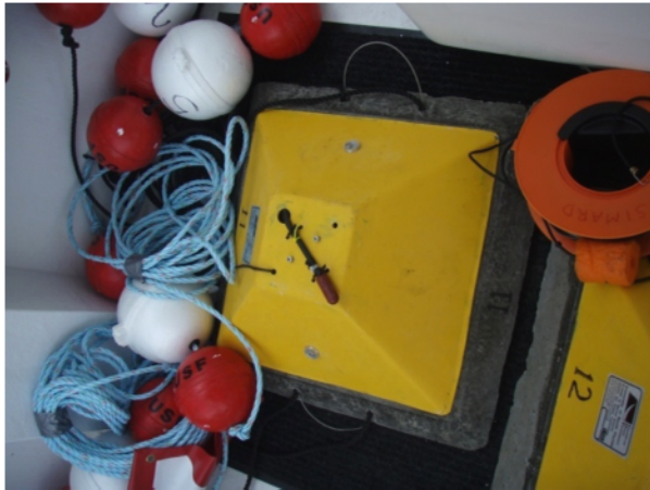
Figure 5. DSG in trawl resistant housing showing hydrophone coming out of the top. The base is made of cement that nestles inside of the pyramidal mount.
