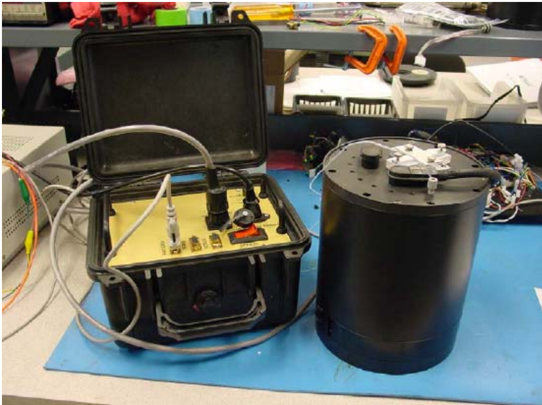
Figure 4. The “Gen 4” Prototype MarChem Analyzer configured for NRL flow immunosensor capability with the external integrated face sealing coupon holder and the laser-based fluorescence detection of the CY-5 fluorophore.
