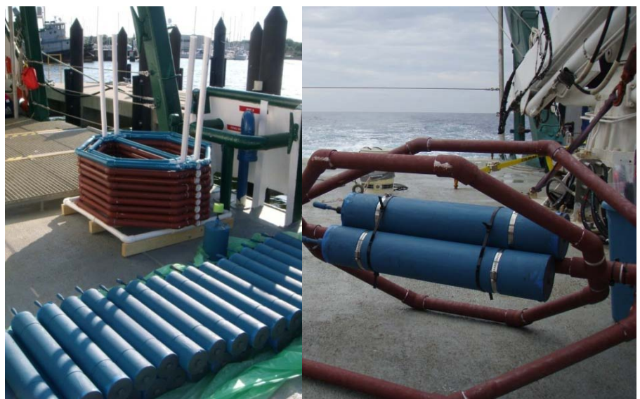
Figure 7. 92 DSG recorders with hydrophones prior to deployment at 63 stations on the West Florida Shelf from the R/V Weatherbird II. The PVC mooring (maroon) had one or two DSG recorders mounted to the center post (right).
