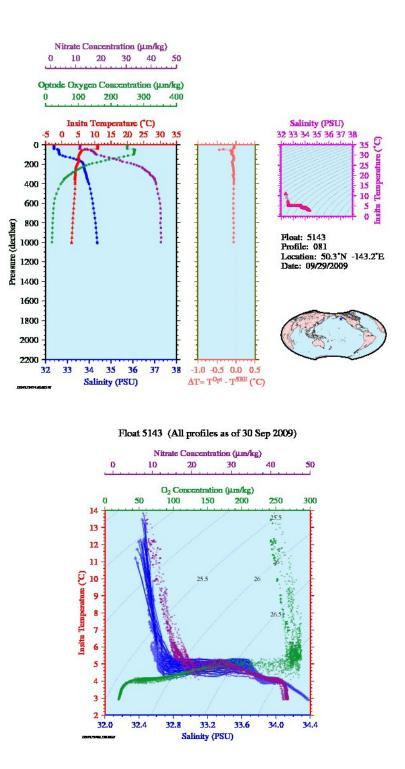
FIGURE 4. Top panel: Temperature, salinity, dissolved oxygen, and nitrate data from 81 profiles from UW profiling float number 5143 in the Northeast Pacific. The profiles were collected at 5-day intervals between August 2008 and September 2009 (the float continues to function normally through the end of 2009). Bottom panel: Salinity, dissolved oxygen, and nitrate plotted as functions of temperature from float 5143.
