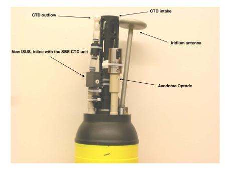
FIGURE 2. The upper endcap of a profling float with the newly designed inline ISUS unit. This float was recently deployed at the HOT site near Hawaii.
