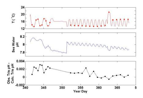
**Figure 3.** Data collected by the SAMI-pH sensor in a variable temperature water bath. The sensor sampled seawater hourly and a tris CRM every day. The temperature during the tris measurement is indicated by the red circles. The pH offset is the difference between the sampled tris and the calculated pH based upon the temperature relationship provided by Andrew Dickson.
