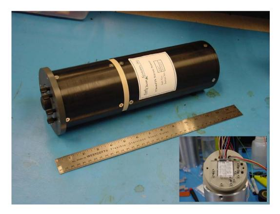
Figure 1. SubChem Systems's compact design for ChemFIN<sup>™</sup> the next generation chemical sensing payload for AUVs, Gliders and Profilers. The ChemFIN compact microfluidics module is also shown (inset).
