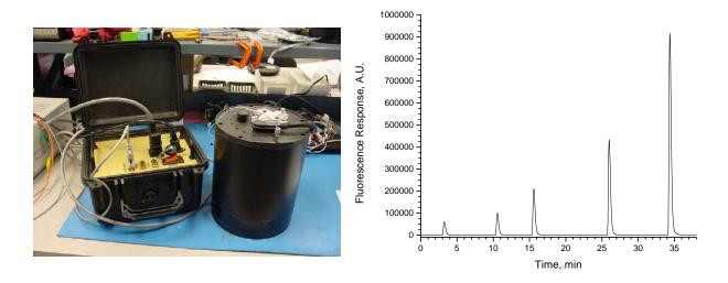
Figure 2. The MarChem Analyzer (left) configured for NRL displacement – based immunoassay with the external integrated face sealing coupon holder and the laser-based fluorescence detection of the CY-5 fluorophore. Shown on the right is the fluorescence response versus time for the successive injection of five 100 μl samples of Cy-5 dye ranging in concentration from 25 to 250 ppb through the system.
