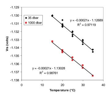
Figure 1. ISFET pH sensor output voltage Vrs (voltage reference to source) is plotted versus temperature for measurements near ambient pressure and at 1000 dbar pressure (equivalent to approximately 1000 m depth in the ocean). There is no significant difference in slope.
