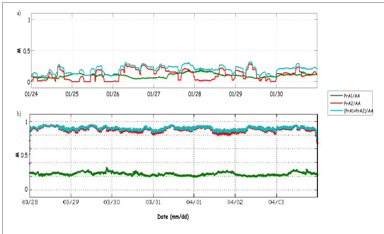
Figure 3. Index of communication masking ( M ) for North Atlantic right whales while a) producing gunshots and b) producing up-calls. The x-axis displays the dates, and the y-axis displays the Masking Index on a scale from 0 to 1. The green line indicates the level of masking under current ambient noise conditions ( PrA1 ) as compared to historic conditions ( AA ), the red line indicates the level of masking induced by vessel traffic ( PrA2 ), and the blue line indicates the level of masking from both ambient and anthropogenic noise combined ( PrA1+PrA2 ). Source levels for up-calls are nearly 40dB lower than for gunshots, therefore communication masking is much higher when right whales are producing up-calls.
