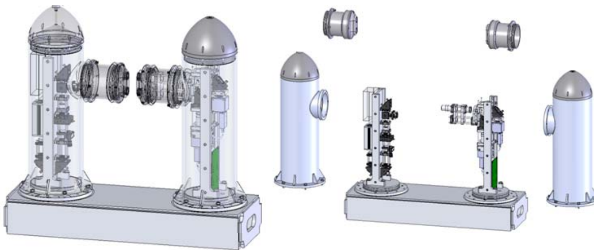
Figure 1. Mechano-optical design of the in-situ HOLOCAM. Design allows simplified field disassembly for service and optical alignment. Technical details are omitted due to proprietary design.
