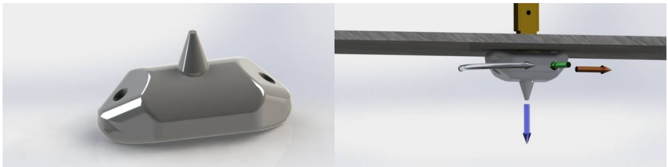
Fig. 6. Computer model of earlier tag model AM-240A (left image) and force sign convention used for reporting the results (right image). Flow is from left to right. The blue, red, and green arrows indicate, respectively, positive lift drag and side forces. The clear arrow indicates positive rotation angle.
