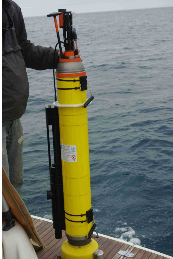
FIG. 1. Biogeochemical float with optics suite attached to side and irradiance sensor on top.
