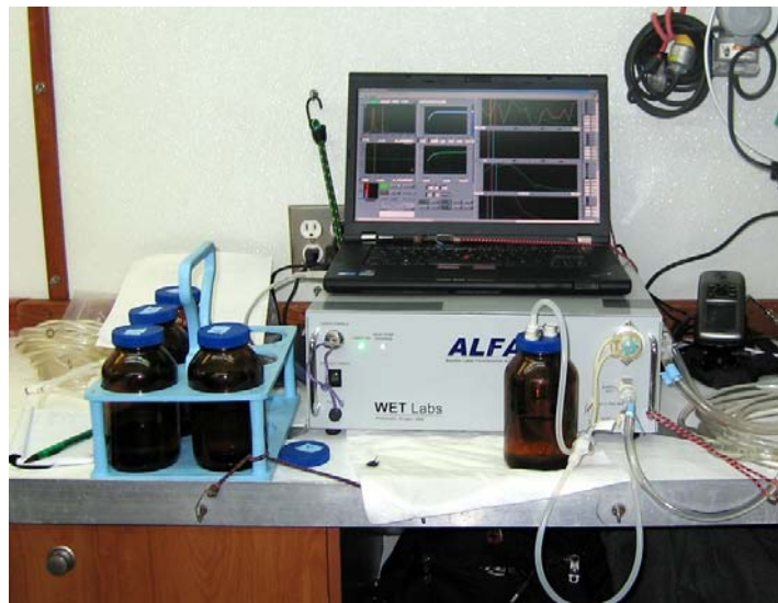
Fig. 5. Upper: a map of transect and station ALFA measurements in the Gulf of Mexico in Apr.-May 2012. Lower: the ALFA-X-405/514 instrument upgraded with a new laser and sampling pump was tested for discrete sample analysis and underway measurements during this deployment.
