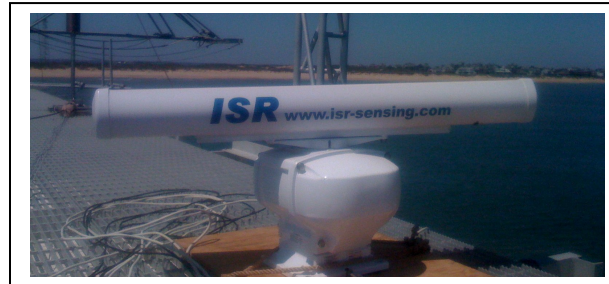
Figure 1. ISR coherent marine radar used for wave sensing.
