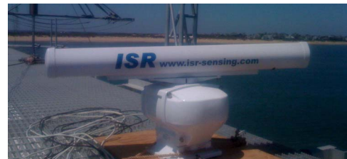
Figure 1. ISR coherent marine radar used for wave sensing.
