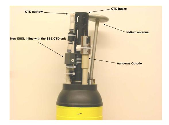
FIGURE 2. A photo of the upper endcap of a profling float with the newly designed inline ISUS unit.
