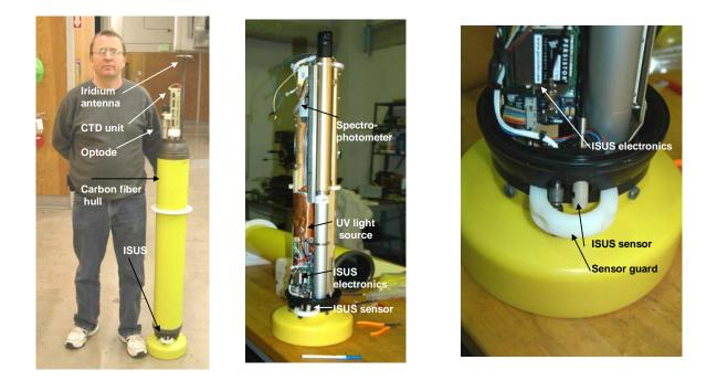
FIGURE 1. The initial design of ISUS for a profiling float. In this version the sensor is located on the lower endcap of the float. The float is also equipped with an Aanderaa Optode dissolved oxygen sensor and uses Iridium communications.
