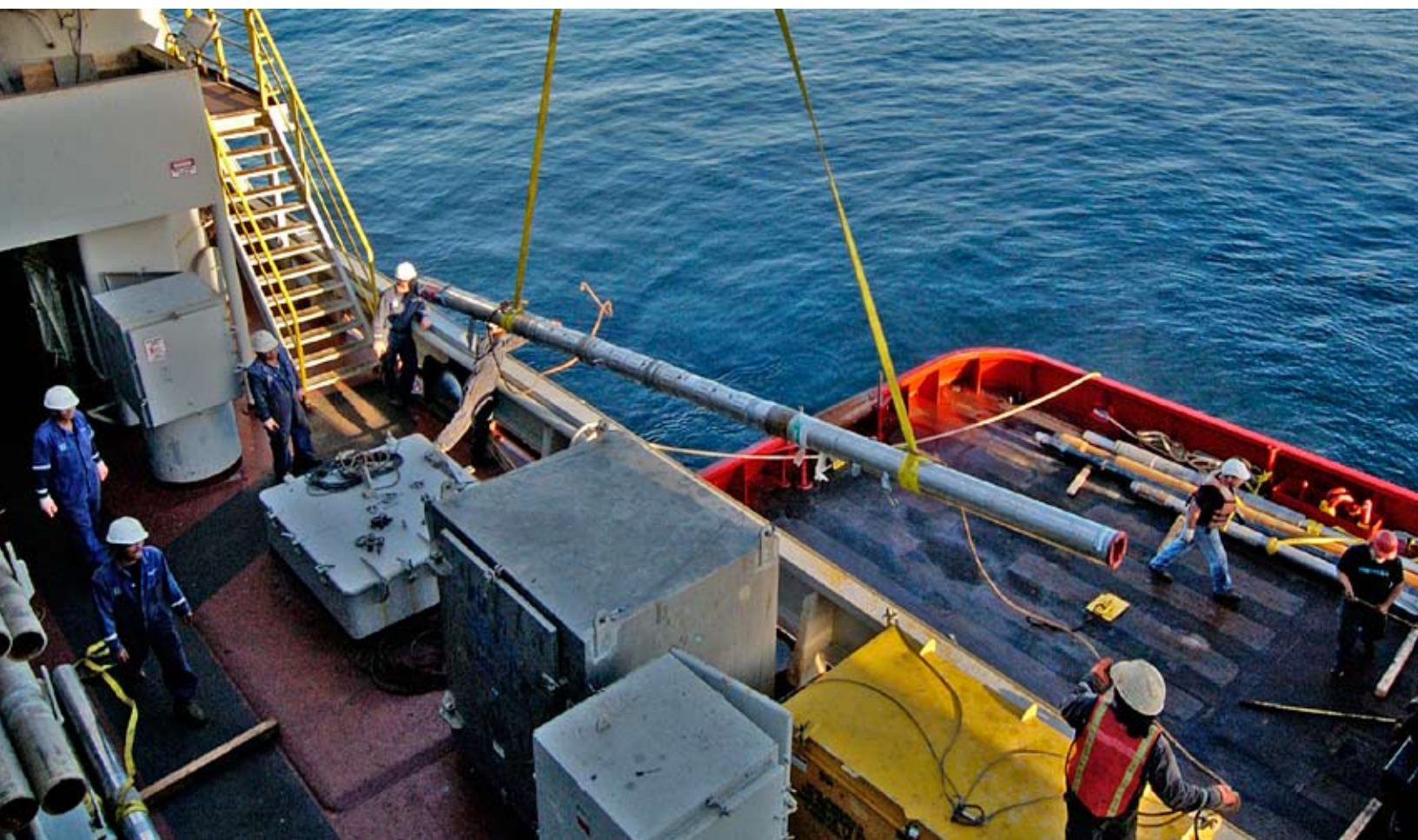
Crew members load drill pipe aboard the scientific drilling vessel Joides Resolution .
