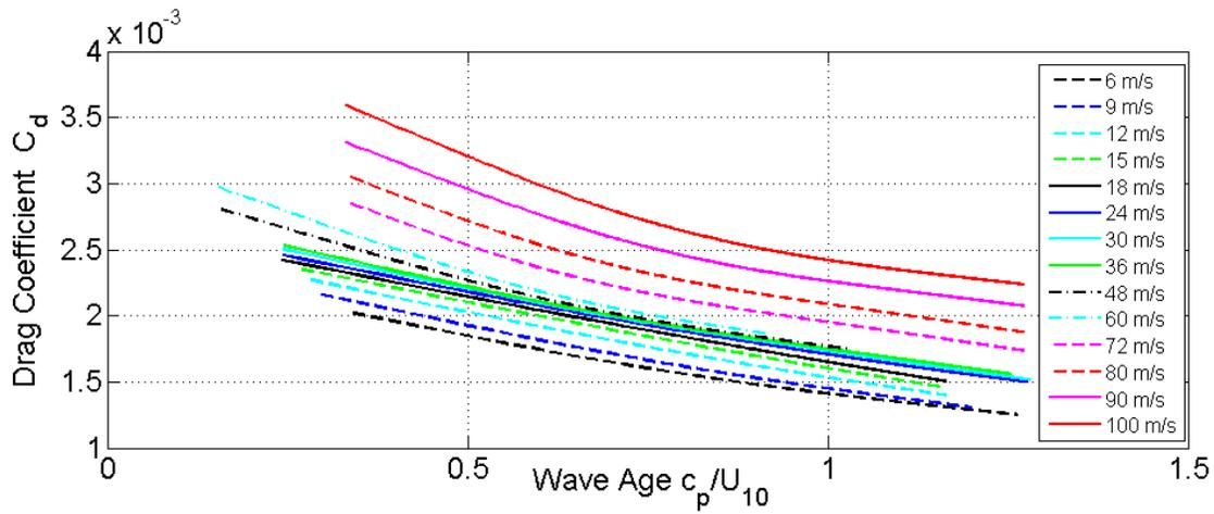
**Figure 1.** Drag coefficient  $C_d$  computed from the modeled wave-coherent wind stress, the tangential viscous stress and the additional wind stress due to separation over breaking waves, as a function of the wave age  $c_p/U_{10}$ .
