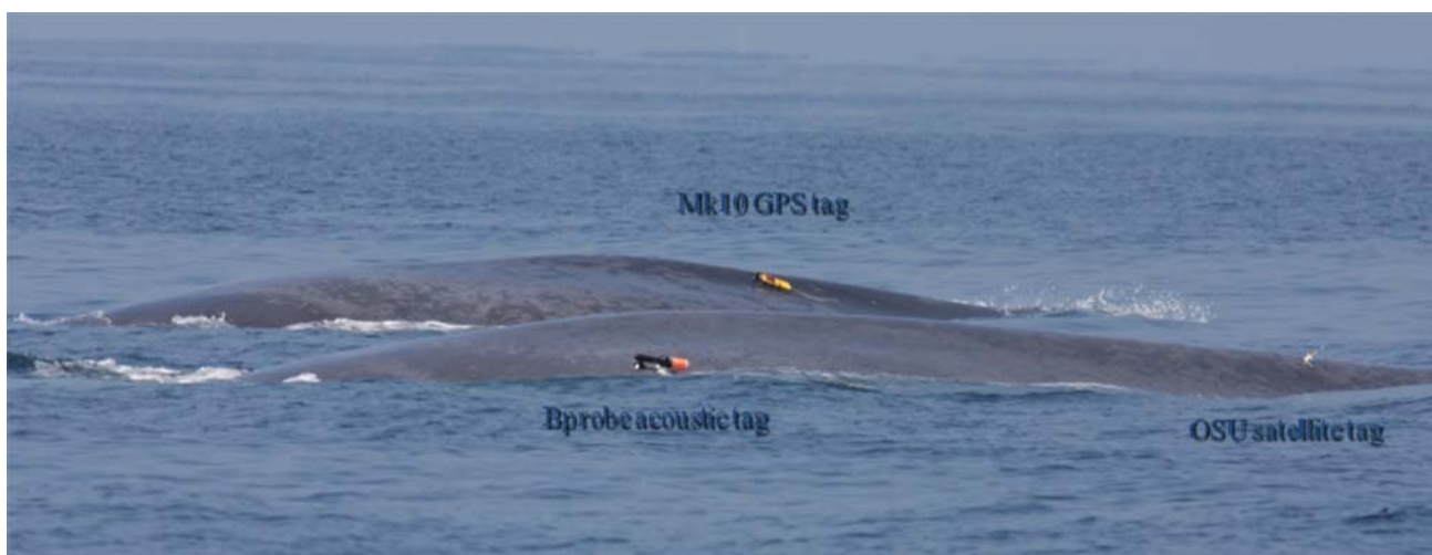
Figure 1. Two blue whales in the Santa Barbara Channel shipping lanes on 16 August 2008 showing three different tag types to be used in this study (suction cup attached Mk10 Fastlock GPS tag and Bprobe and implanted OSU satellite tag.
