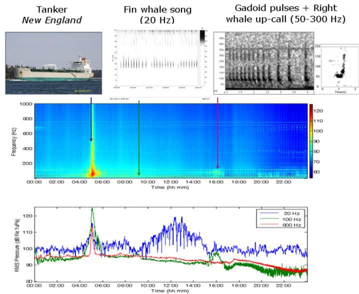
**Figure 2.** Long-term spectrogram and received levels over time for select  $1/3^{\text{rd}}$  octave frequency bandwidths from a single ARU location on 27 December 2007. Note peaks in received levels associated with a transiting commercial vessel and vocalizing whales and fish.
