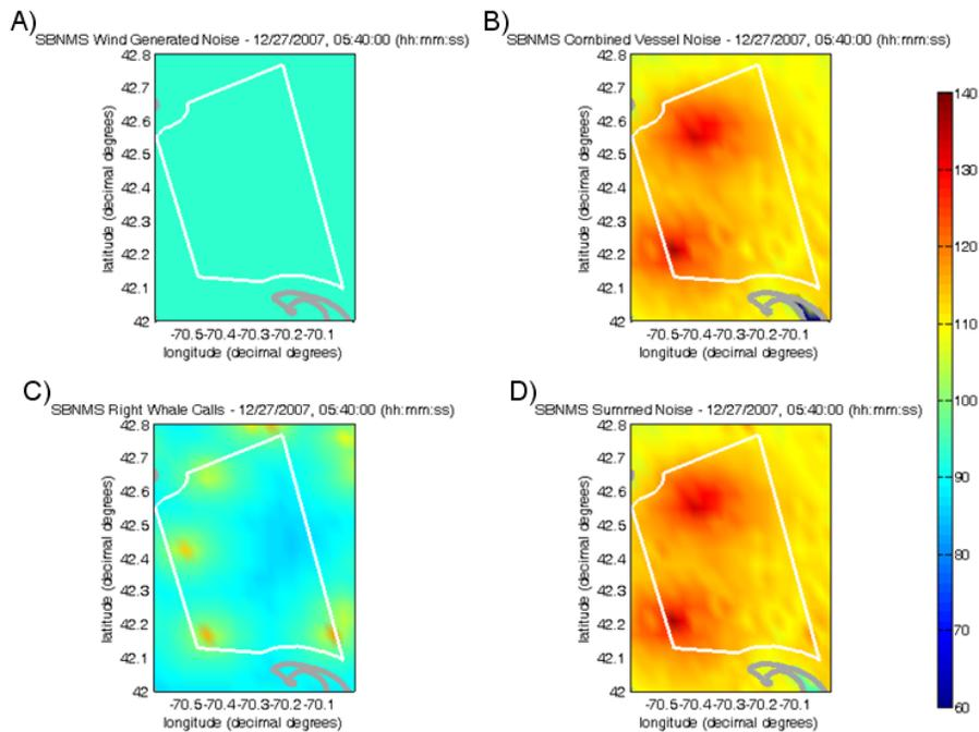
**Figure 4. Spatial distributions of noise levels as contributed by A) wind, B) large commercial vessels, and C) up-calling right whale, and D) a summation of wind, vessels and whales. Noise levels were predicted by AIM for the 100Hz 1/3<sup>rd</sup> octave frequency band using empirical data from a 10-minute sample (05:40 - 05:50L) on 27 December 2007. Noise level intensities (dB re 1µPa) are scaled according to the legend on the right.**
