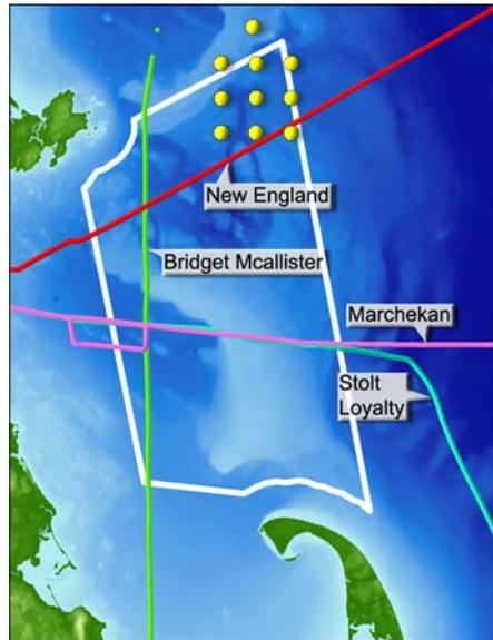
**Figure 1.** Plot of all AIS-tracked large commercial vessel traffic in the sampling region on 27 December 2007. Empirical data from the ten ARUs (yellow dots) were used to calculate vessels' source levels in AIM.
