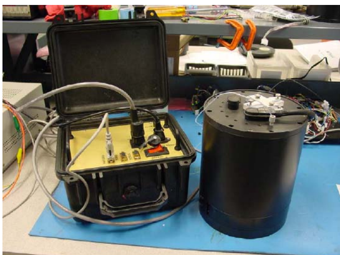
Figure 3. The MarChem Analyzer (left) configured for NRL displacement – based immunoassay with the external integrated face sealing coupon holder and the laser-based fluorescence detection of the CY-5 fluorophore. The system is also shown (right) configured for submerged deployment from the URI-GSO Pier in Narragansett Bay.
