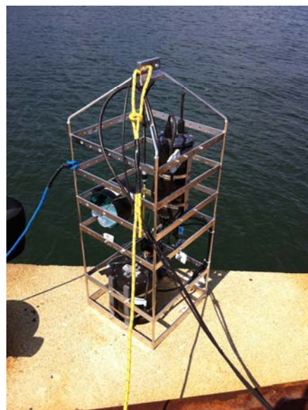
Figure 3. The MarChem Analyzer (left) configured for NRL displacement – based immunoassay with the external integrated face sealing coupon holder and the laser-based fluorescence detection of the CY-5 fluorophore. The system is also shown (right) configured for submerged deployment from the URI-GSO Pier in Narragansett Bay.
