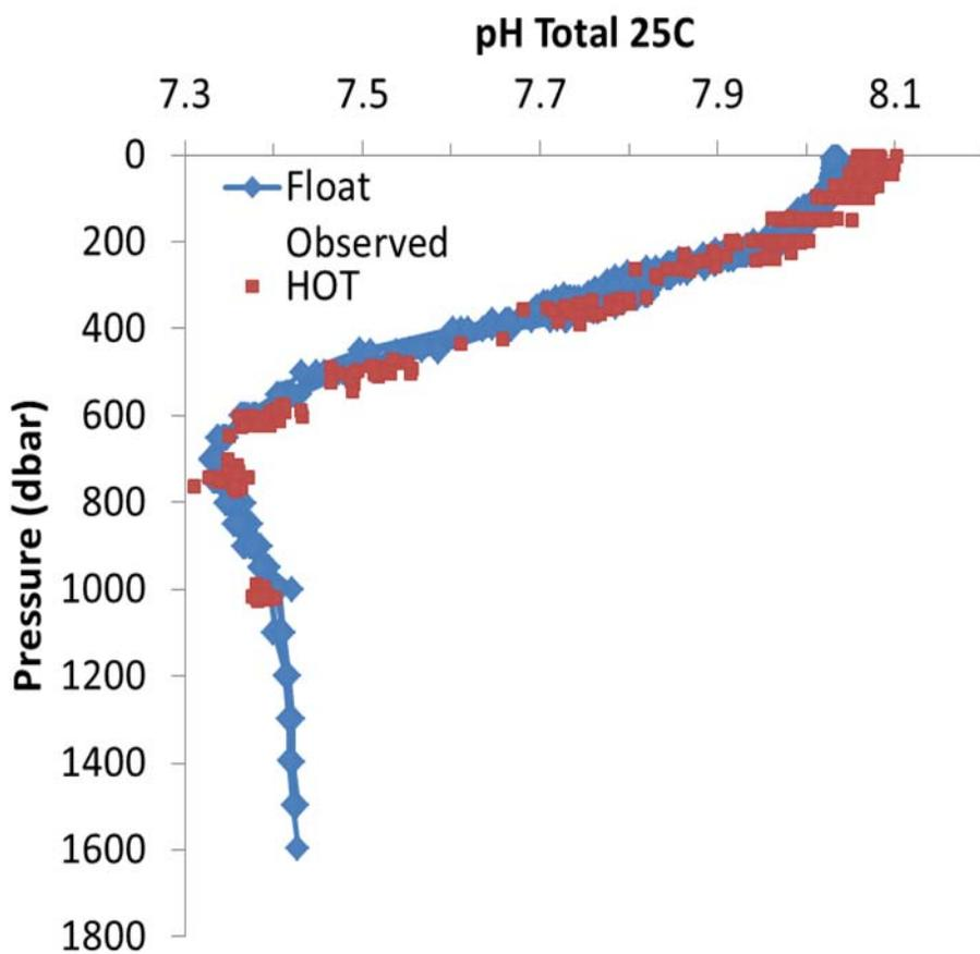
Fig. 2. pH values measured with the Deep-Sea Durafet mounted on a CTD/rosette sampler (solid lines) and pH values measured spectrophotometrically using m-cresol purple indicator in samples collected with the rosette (dots) at four stations off Southern California. Measurements made by Todd Martz and Yui Takeshita (SIO).
