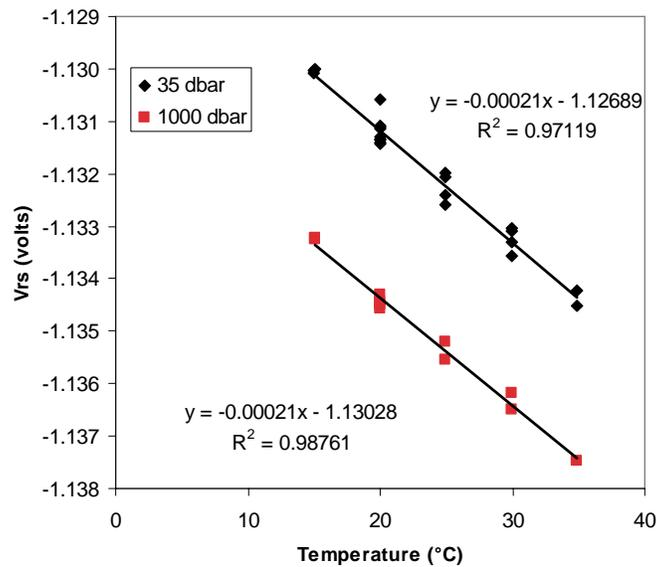
**Figure 1. ISFET pH sensor output voltage  $V_{rs}$  (voltage reference to source) is plotted versus temperature for measurements near ambient pressure and at 1000 dbar pressure (equivalent to approximately 1000 m depth in the ocean). There is no significant difference in slope. Measurements were made in 0.01 mol/l HCl.**
