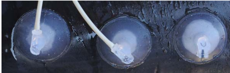
Figure 2. Top panel shows three DTAG3 cups at the time of application. Note peripheral air pockets in addition to the central bubble. Bottom panel 14 minutes later. The peripheral bubbles have coalesced into the central bubble. Where the central bubble margin is irregular in the top panel, that irregularity is preserved at the later time.
