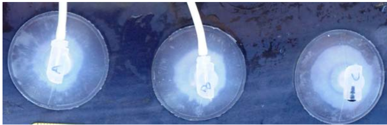
Figure 2. Top panel shows three DTAG3 cups at the time of application. Note peripheral air pockets in addition to the central bubble. Bottom panel 14 minutes later. The peripheral bubbles have coalesced into the central bubble. Where the central bubble margin is irregular in the top panel, that irregularity is preserved at the later time.
