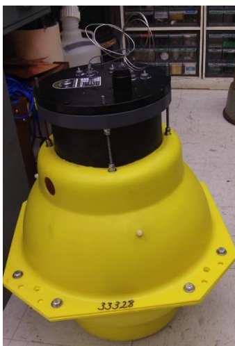
Figure 1. Submersible, battery-powered system for in-situ ammonium measurement in natural waters (currently in final assembly).
