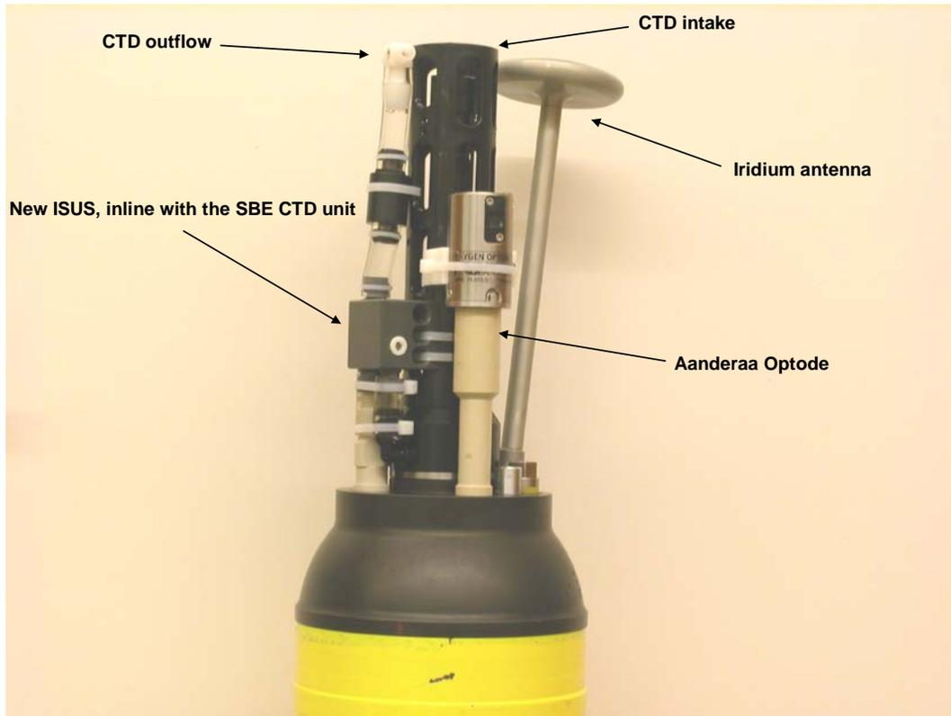
**FIGURE 2.** A photo of the upper endcap of a profiling float with the newly designed inline ISUS unit.
