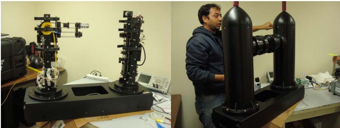
Figure 1. Internal electro-optical structure of the first in-situ HOLOCAM prototype (left panel). Pressure housings being assembled onto the HOLOCAM (right panel).
