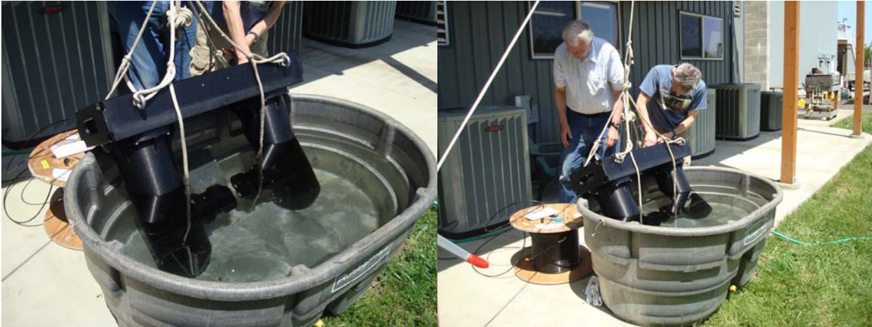
Figure 2. Submersion and system testing of the HOLOCAM at WET Labs.
