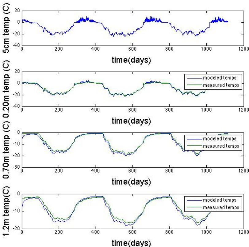
Figure 3. Measured and modeled ground temperatures at the Drew Point USGS meteorological station. 5 cm soil temperatures (top panel) were model input data; modeled temperatures at depth are plotted along with measured temperatures in lower three panels.
