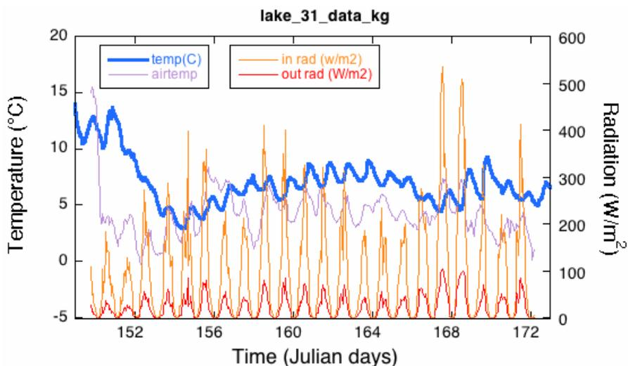
Figure 2. Example of water temperature, air temperature, and solar radiation at Lake 31, spanning a late summer storm between Julian days 150-155. Note the dramatic drop in lake temperatures, possibly due to mixing of colder waters by wind energy.
