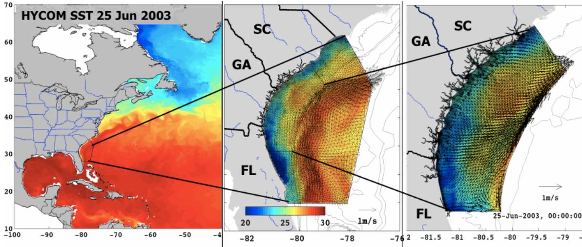
**Figure 2:** UNC-SAB modeling system sequence that nests the regional-scale QUODDY implementation (middle) within the 1/12 deg operational HYCOM-GODAE model (left). The limited-area QUODDY implementation (right) includes the estuary and tidal inlets along the Georgia/South Carolina coast and extends to the shelf-break.
