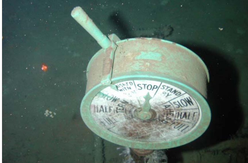
Figure 1: Telegraph from the bridge of the Robert E. Lee standing up right on the seafloor, 200 feet way from the main shipwreck structure.
