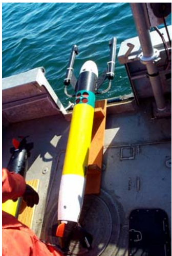
Figure 1. Deployment of VPR-REMUS in coastal waters off Woods Hole.
