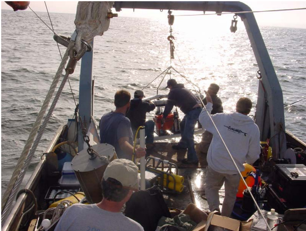
Figure 2. Scientists on the stern of the R/V Shana Rae recovering a battery-powered mooring that had been placed on the bottom in Monterey Bay for a 2 week time-period to test the performance of three different types of autonomous submersible chemical analyzers, including the APNA III.
