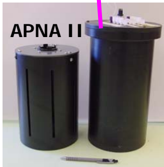
Figure 1. The IOPC profiler with the APNA II nutrient analyzer payload ready for deployment in Monterey Bay from the R/V Shana Rae and examples of hourly profiles for nitrate (blue), chlorophyll (green), and density (black) that were obtained autonomously with the system in Monterey Bay.
