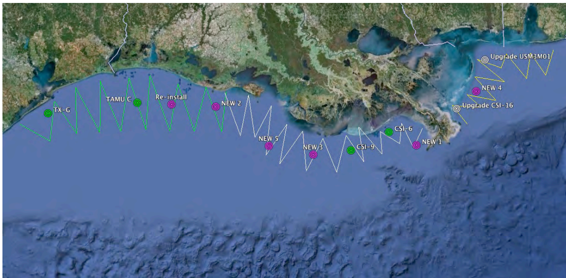
Figure 6. Hypoxia monitoring plan for the Gulf shelf; additional plans are under development for the estuaries and nearshore environment with the Gulf of Mexico Alliance Water Quality and Nutrient Reduction Priority Issue Teams.
