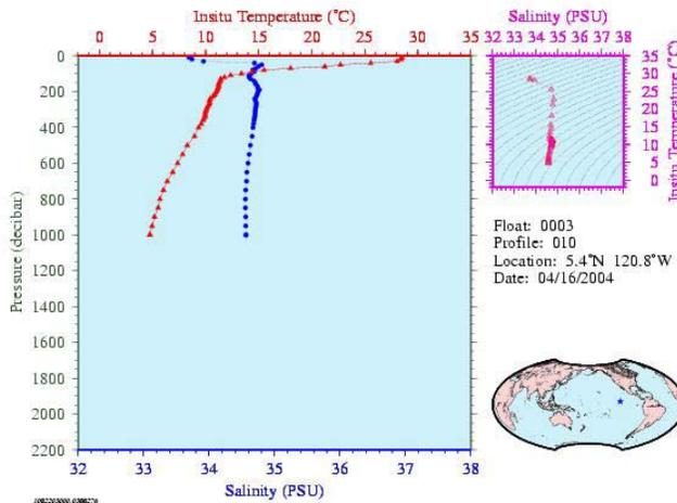
**Figure 2.** Top left: The head of a Webb/Apex float, showing a SeaBird CTD unit and a broadband hydrophone for an acoustic rain gauge. Top right: A profile from UW ARG float 0003, deployed in the eastern Equatorial Pacific in January of 2004 (the inset shows the float location). Bottom panel: Wind speed and rainfall measured from ARG float 0003, while the float was drifting at a depth of 1000 m in the eastern Equatorial Pacific. Note the episodic nature of the tropical rainfall events.
