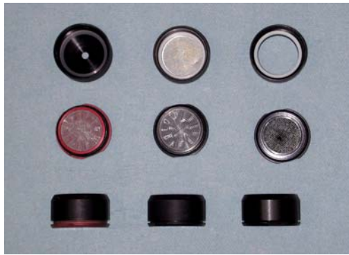
Figure 1. ESP “pucks” that hold 25 mm user-defined media. Pucks are highly configurable for performing different types of analyses, but all conform to a common outer envelope (bottom row). The three pucks shown (one puck per column shown assembled in bottom row with top and bottom halves above) are used for (left to right) creating cell homogenates, archiving cells for microscopy, and developing DNA probe arrays. All utilize a common core processor, the ESP, for carrying out those functions. Pucks are stored in rotating carousels and loaded/unloaded into the sample collection and processing system using a mechanical actuator.
