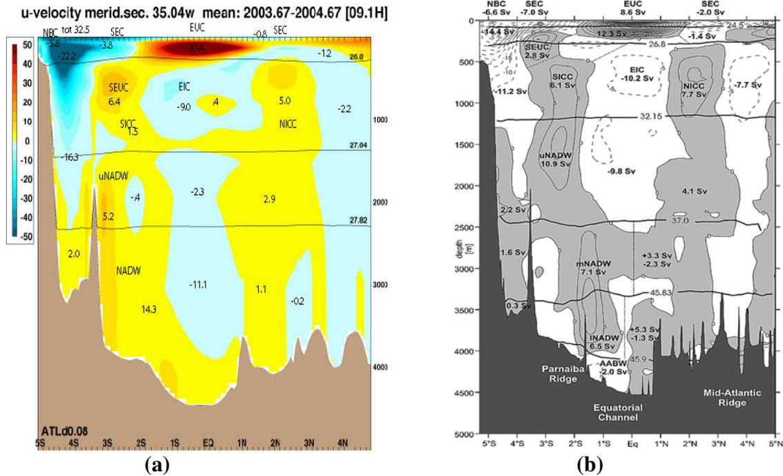
**FIGURE 2.** (a) A vertical section of the mean velocity across  $35^{\circ}\text{W}$  from  $5^{\circ}\text{S}$  to  $5^{\circ}\text{N}$  from the  $1/12^{\circ}$  Atlantic system. The mean is over the time period July 2003 through August 2004. (b) Observations of transports across  $35^{\circ}\text{W}$  (from Schott et al., 2003)
